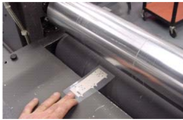
b) Transfer the preform to the part by applying heat and pressure.
